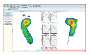
Film of the step sequence with simultaneous display of force, surface and pressure curves.
