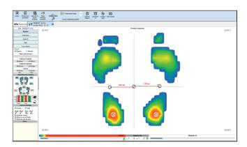
Centers of pressure and maximum pressure for each foot, front and rear D/G distribution and by zone, projec tion of the center of gravity, study zone, film of the static.
