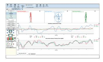
Stabilometry: ellipses and dimensions of centers of thrust. Oscillation and % in area and time: frontal and sagittal plane. Parameterizable in duration, frequency, % of points.
